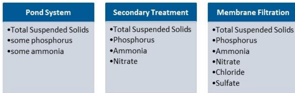
Figure 1-3 General types of treatment systems and the pollutants they remove
